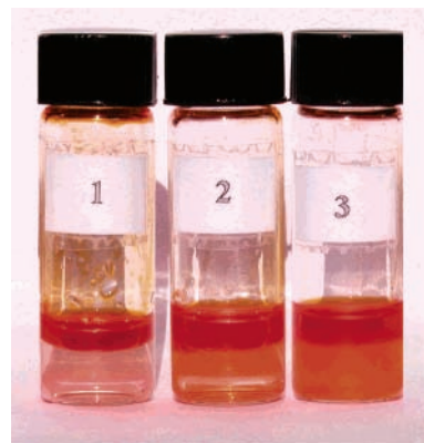
Figure 3. Orange OT partitioning experiment in hexane equilibrated with MeOH/H 2 O (1:1) after 12 h. Vial 1 has no additive, vials 2 and 3 have NaDC 7 (48 mM) and tetramer 2 (12 mM), respectively.
